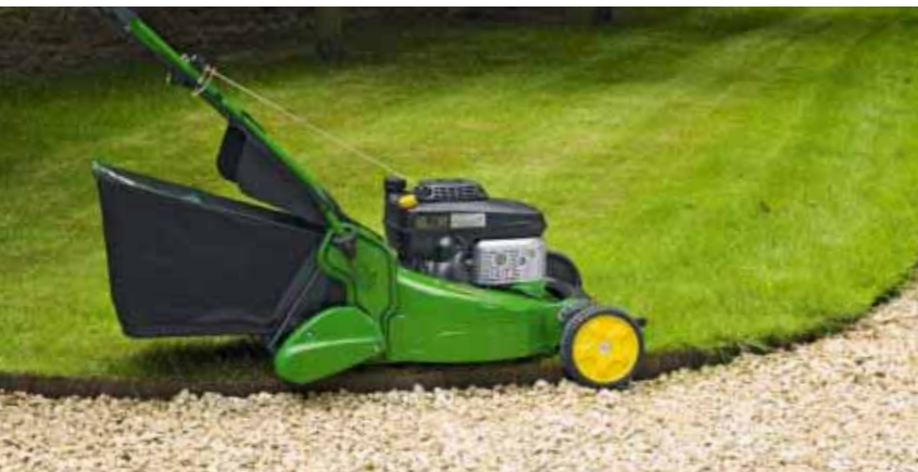
The rear roller protects against scalping when mowing the edge.
