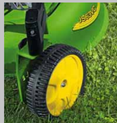
Front caster wheels on the JS63VC turn for outstanding manoeuvrability along contoured landscaping and tight corners.
